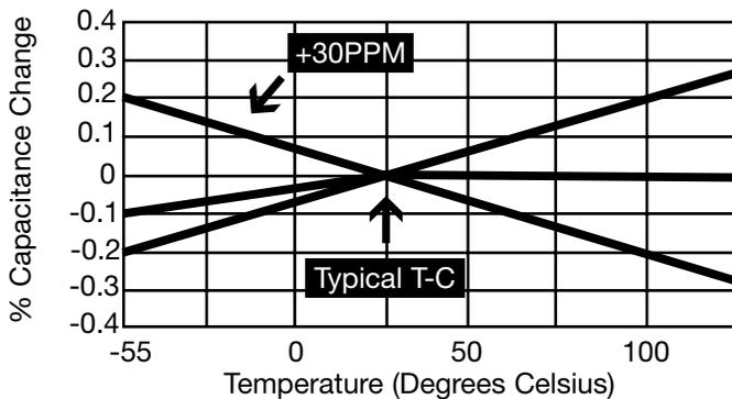
**Typical X7R Temperature Coefficient**
