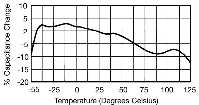
X7R ceramics, Class II, are the most temperature-stable ceramics in their class. Capacitance for X7R varies under the influence of electrical operating conditions such as voltage and frequency. It also varies with time, approximately 2.5%  $\Delta\text{C}$  per decade hour, representing about 12.5% change in ten years.
